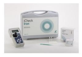
Acidic environment reduces ferric iron (Fe<sup>3+</sup>) to ferrous iron (Fe<sup>2+</sup>) which reacts with bathophenanthroline. The resulting red complex of iron and bathophenanthroline correlates with iron concentration and is measured at 525 nm with the iCheck device. The measurement range of iCheck Iron is 1.5 – 12.0 mg/L.
