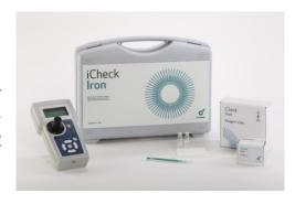
Iron quantification is based on a colorimetric reaction with bathophenanthroline. The resulting red complex correlates with iron concentration and is measured at 525 nm with the iCheck device. The measurement range of iCheck Iron is 1.5 – 12.0 mg/L.
