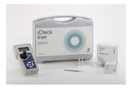
Iron quantification is based on a colorimetric reaction with bathophenanthroline. The resulting red complex correlates with iron concentration and is measured at 525 nm with the iCheck device. The measurement range of iCheck Iron is 1.5 – 12.0 mg/L.
