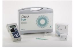
Acidic environment reduces ferric iron (Fe<sup>3+</sup>) to ferrous iron (Fe<sup>2+</sup>) which reacts with bathophenanthroline. The resulting red complex of iron and bathophenanthroline correlates with iron concentration and is measured at 525 nm with the iCheck device. The measurement range of iCheck Iron is 1.5 – 12.0 mg/L.
