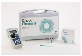
algorithm calculates vitamin A concentration in mg retinol equivalents (RE) per kilogram (mg RE/kg). The measurement range of iCheck Chroma 3 is 3.0 – 30.0 mg RE/kg.
