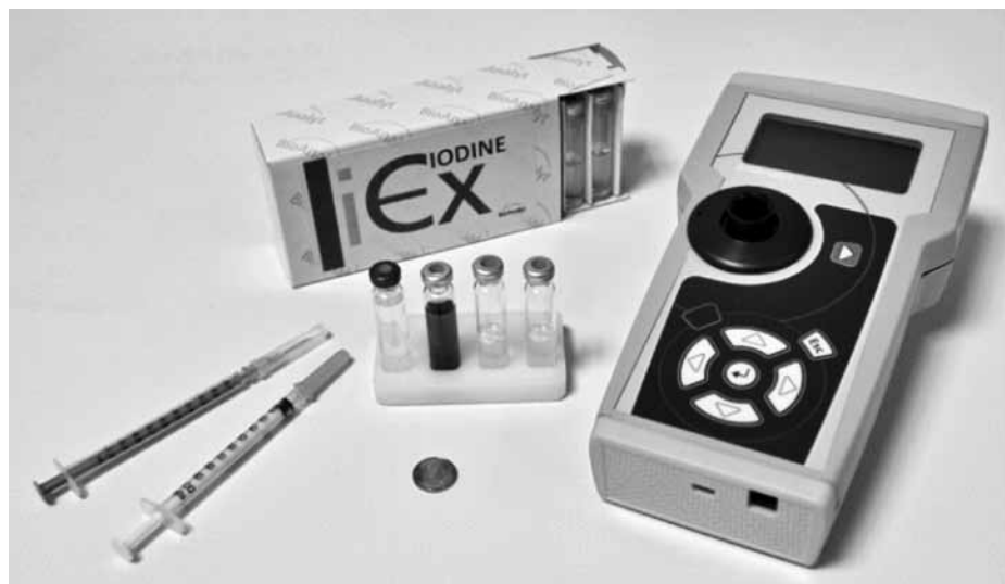
FIG. 1. Prototype of the portable device that has been validated as described in this paper. As an indication of size, a 1-cent Euro coin has been placed in the picture
