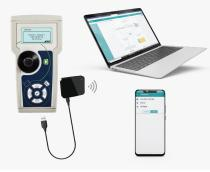
iCheck Connect is a free companion web and mobile app. Data can be transferred from your iCheck device via a USB cable or wireless Bluetooth adapter. iCheck Connect can support analysis by:
